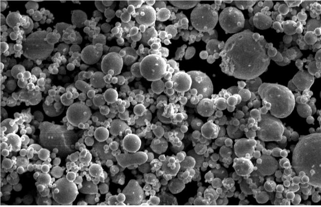
Figure 2: SEM image of fine gas atomised powder
