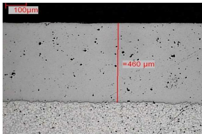
Figure 6: Cross section of ferritic stainless steel coating applied by High pressure cold spray by obz innovation gmbh.
