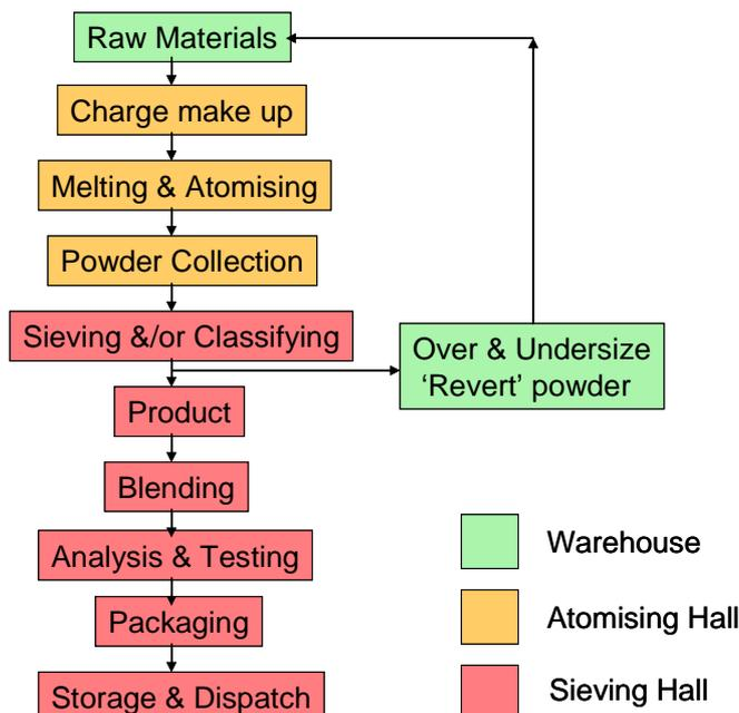
Figure 1: Flow diagram of the gas atomisation process
