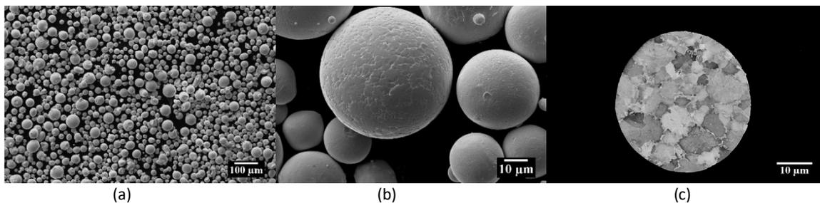
SEM micrographs of Osprey® 2507 a) -53 +15 µm powder with a spherical morphology, b) smooth surface and low level of powder satellites and c) micrograph of powder in cross-section, in back scattered electron mode, highlighting the fine cellular structure.
