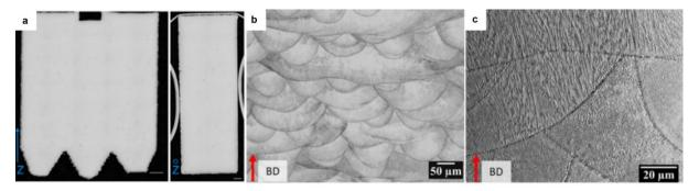
LOM micrographs, a) a low magnification profile of the cross-section along build direction and normal to build direction, b) chemically etched cross-section showing traces of the melt pools, c) higher magnification micrograph showing the ultrafine cellular/dendritic solidification structure.
