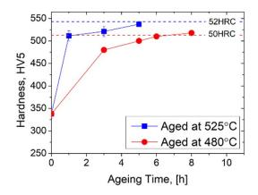
Hardness after ageing at 480°C and 525°C vs. time for samples directly aged.
