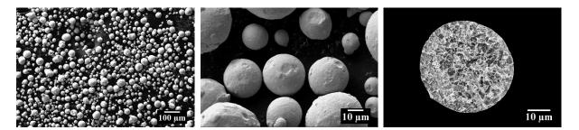
SEM micrographs of a) -53 +15 µm powder with spherical morphology, b) smooth surface and low level of powder satellites and c) micrograph of powder in cross-section, in back-scatted electron mode, highlighting the fine cellular structure.
