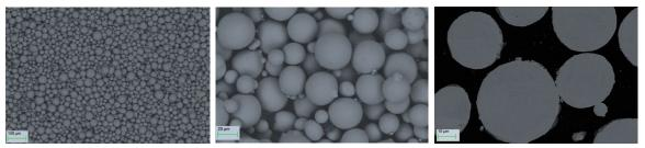
SEM micrographs of -63 +20  $\mu$ m powder with a spherical morphology (HS Circularity 0.95), smooth surface and low level of powder satellites (magnifications x100 & x250) and a section through the powder (magnification x1000), with no visible internal porosity.
