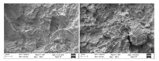
SEM micrographs of Osprey<sup>®</sup> TI-6AL-4V L-PBF material in a heat-treated condition (left) and HIP material (right), both featuring ductile fracture surfaces.
