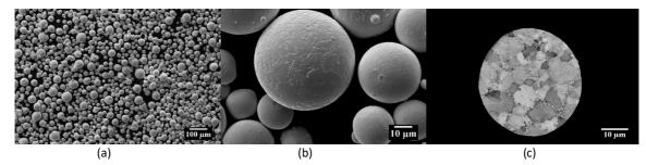
SEM micrographs of Osprey<sup>®</sup> 2507 a) -53 +15 µm powder with a spherical morphology, b) smooth surface and low level of powder satellites and c) micrograph of powder in cross-section, in back scatted electron mode, highlighting the fine cellular structure.
