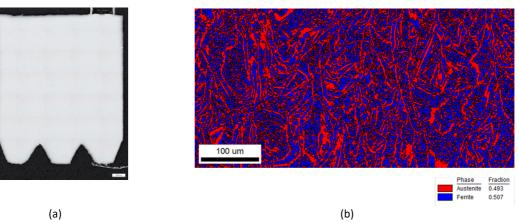
Micrographs of Osprey<sup>®</sup> 2507 a) As-built vertical section of the test specimen with near full dense part with 99,9%+ relative density, b) EBSD image indicating phase balance and microstructure in the material after suitable heat treatment.
