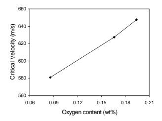
Figure 3: Effect of oxygen content of 316L stainless steel powder on its critical velocity for deposition in cold spraying. Li et al. [4]
