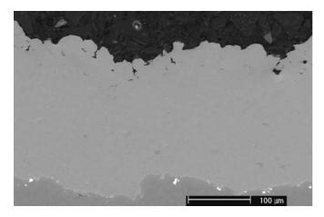
Figure 5: High Pressure cold sprayed (HPCS) Ni-30Cu coating on grit-blasted steel substrate, using -38+16  $\mu$ m gas atomise powder from Sandvik Osprey, Koivuluoto et al. [8]
