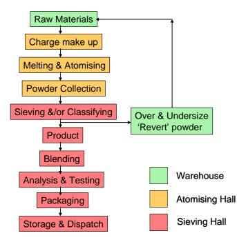
Figure 1: Flow diagram of the gas atomisation process
