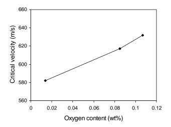
Figure 4: Effect of oxygen content of monel powder on its critical velocity for deposition in cold spraying. Li et al. [4]
