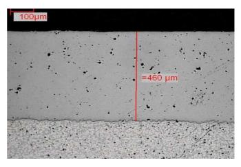
Figure 6: Cross section of ferritic stainless steel coating applied by High pressure cold spray by obz innovation gmbh.
