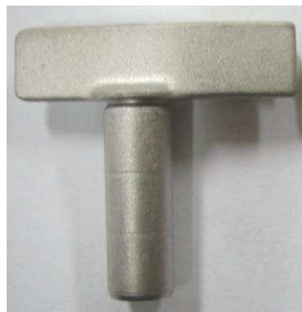
Fig. 1 Example of MIM'ed turbocharger vane.
