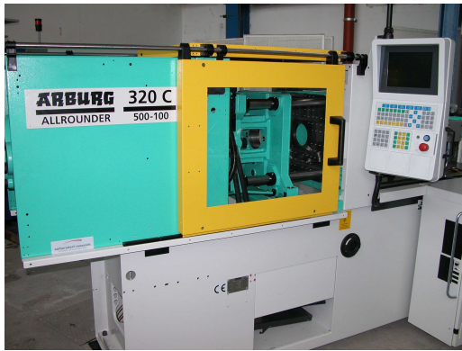
Figure 2. Injection moulding machine used for component fabrication at ARC Seibersdorf research GmbH
