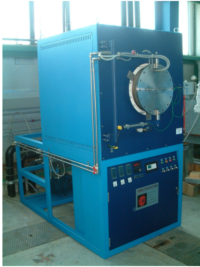
Figure 5. Combined debinding and sintering furnace for maximum temperatures of 1100°C
