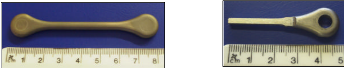
Figure 2. (a) MIM tensile test bar. (b) One half of an as tested machined MIM tensile test bar.
