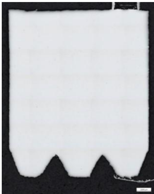
As-built vertical section of the test specimen with near full dense part with 99.9% + relative density As-built vertical section of the test specimen with near full dense part with 99.9% + relative density.
