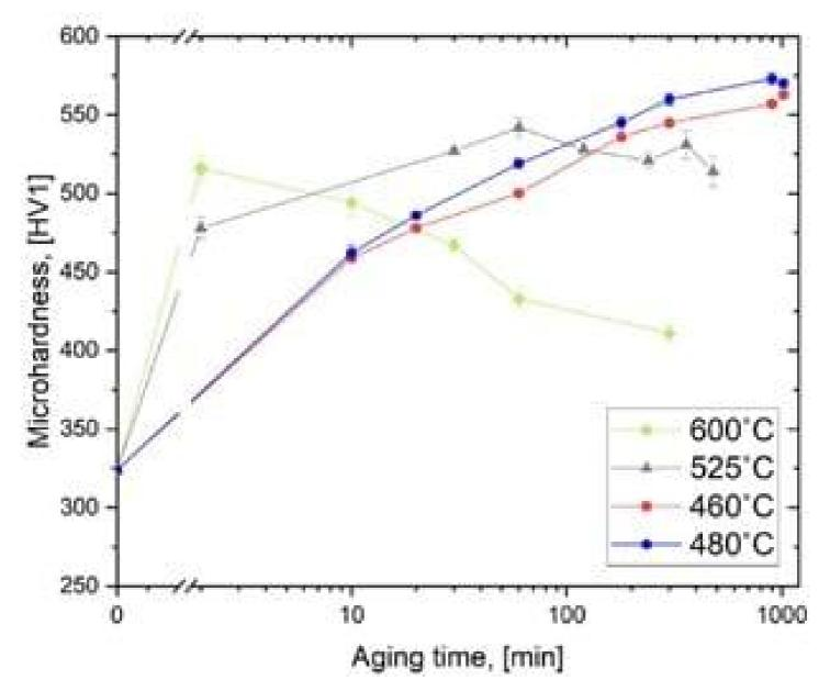
Maximum hardness, approximately 550 HV (53 HRC), is typically reached after a heat treatment at 480°C/896°F for 6–10 hours, depending on the part size. Lower hardness can be achieved by aging at higher temperatures. The use of maraging steels in applications such as die casting tooling might require an aging temperature of approx. 525°C/977°F to achieve an overaged structure to ensure the thermal stability in service.
