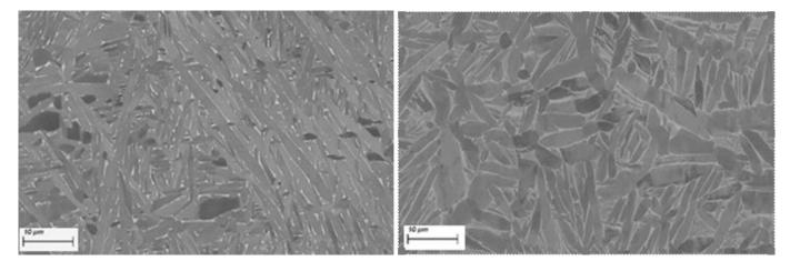
SEM micrographs of Osprey® TI-6AL-4V-ELI (Grade 23) Laser - Powder Bed Fusion (L-PBF) material in a heat-treated condition (solution annealed at 850 °C/1,562 °F for 2h in argon) on the left, featuring a fine lamellar and dense microstructure is identified which originates from the decomposition of martensitic []' as expected; showing a phase transformation that gave rise to a coarser structure consisting of a [] phase matrix (grey) and an interlamellar [] phase
