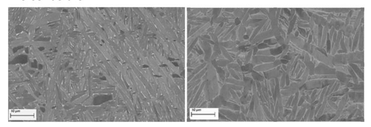
SEM micrographs of Osprey® TI-6AL-4V-ELI (Grade 23) Laser - Powder Bed Fusion (L-PBF) material in a heat-treated condition (solution annealed at 850 °C/1,562 °F for 2h in argon) on the left, featuring a fine lamellar and dense microstructure is identified which originates from the decomposition of martensitic  $\alpha$  as expected; showing a phase transformation that gave rise to a coarser structure consisting of a  $\alpha$  phase matrix (grey) and an interlamellar  $\beta$  phase (bright).
