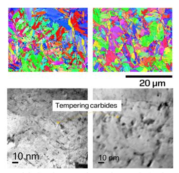
Top left: directly tempered. Top right: Quenched and tempered. Bottom left and right show tempering carbides.
