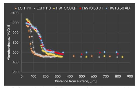
Microhardness profiles after the nitriding process are shown and compared with those of AISI H13 and AISI H11 hot work tool steels.
