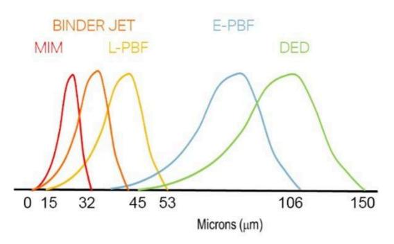
Typical particle size distributions for Additive Manufacturing.
