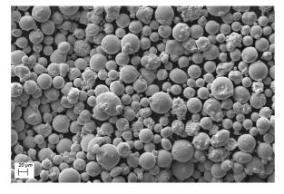
The powder morphology of Osprey<sup>®</sup> 718-AM alloy powder is typically spherical in morphology, with smooth surface and low level of powder satellites.
