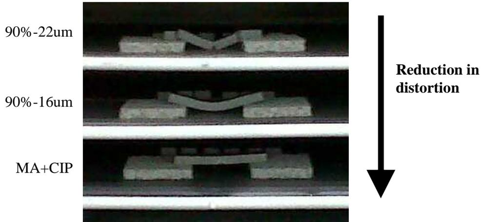
**Figure 8:** Distortion of 4340 following sintering at 1100°C. Powder particle size distributions are indicated alongside images.
