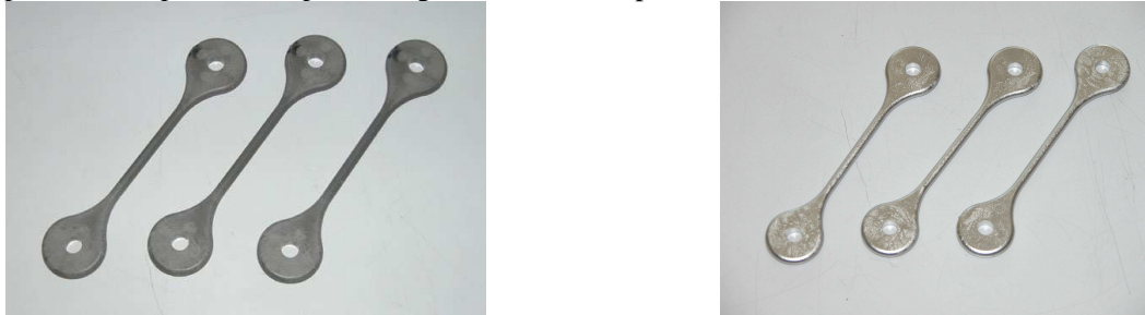
Figure 4. Tensile test specimens before and after sintering.
